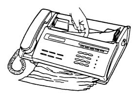
It will release the grip on the document. Wait until the white roller in the unit stops moving. You can then remove the jammed document without damaging your unit. Close the cover. 'DOCUMENT JAM' message disappears and the unit returns to the standby mode.
